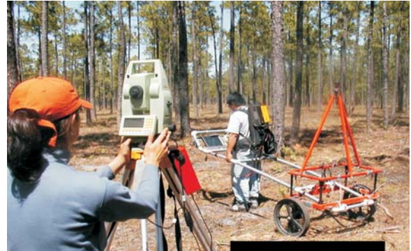
Em61 MKII instrument integrated with a Robotic Total Station for positioning.
