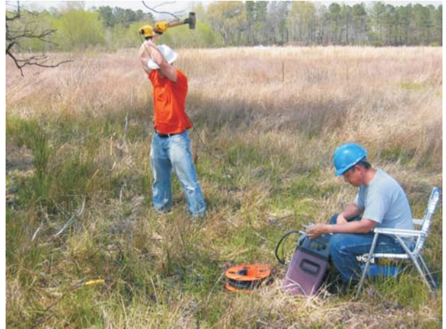
Seismic refraction survey in Dalton, Georgia.
