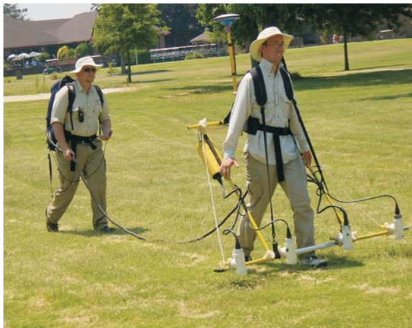
TM-6 Quad Magnetometer system at Langley AFB, Virginia.
