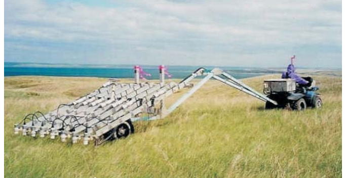
TM-6 Towed Array system.
